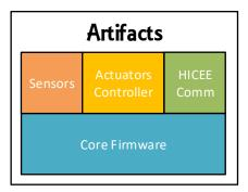
Figure 5.6 - Artefact Embedded Software Architecture.
