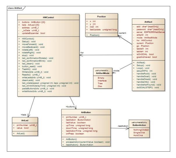
Figure 5.8 - Artefact Embedded Software Class Diagram.
