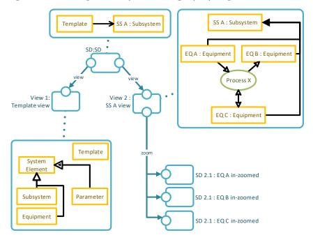
Figure 4.7 - Example of a System Design (SD) Represented in OPM.
