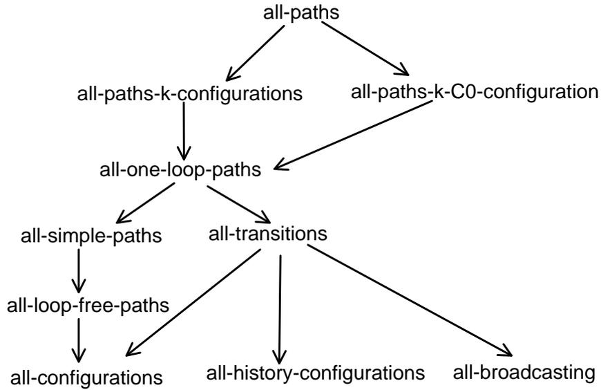
Figure 2.1 - Inclusion relation among the SCCF test criteria considering resettable models
