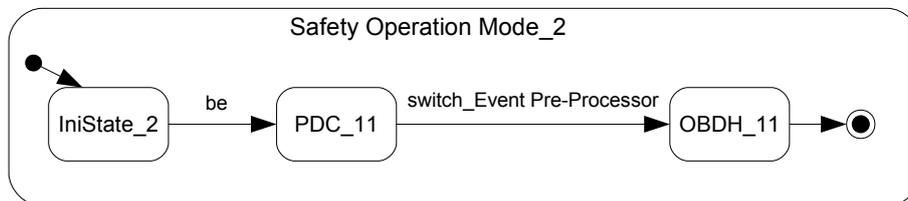
Figure 4.4 - Normal scenario 71: COMPOSITE state *Safety Operation Mode\_2*
