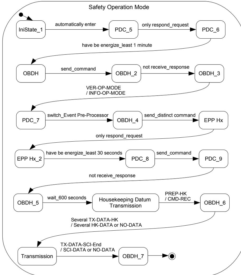
Figure 4.5 - Normal scenario 71: COMPOSITE state *Safety Operation Mode*
