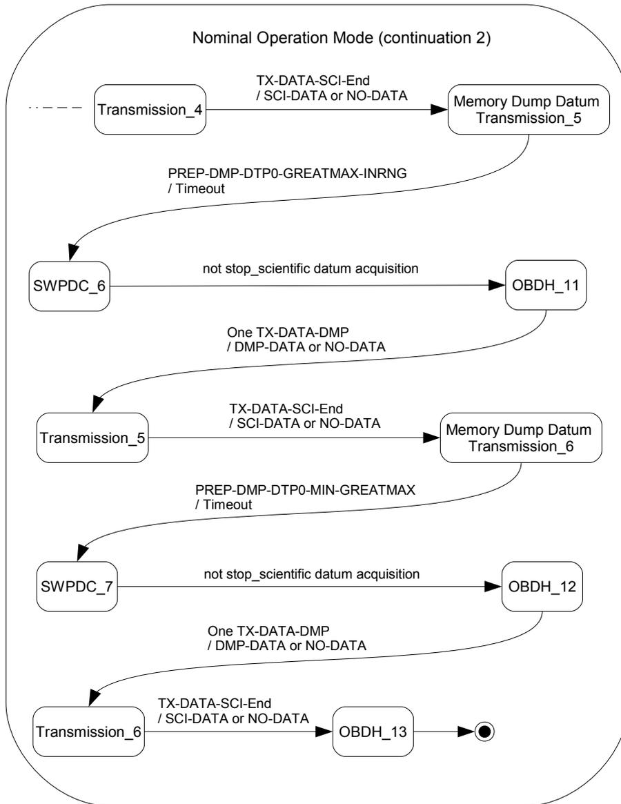
Figure 4.19 - SOLIMVA's unfolded scenario 73.2: *Nominal Operation Mode* (Part 2)
