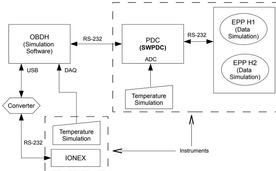
Figure 3.1 - Functional architecture defined for QSEE project. Caption: ADC = Analog-to-Digital Converter; DAQ = Data Acquisition Board; RS-232 = Recommended Standard 232; USB = Universal Serial Bus
