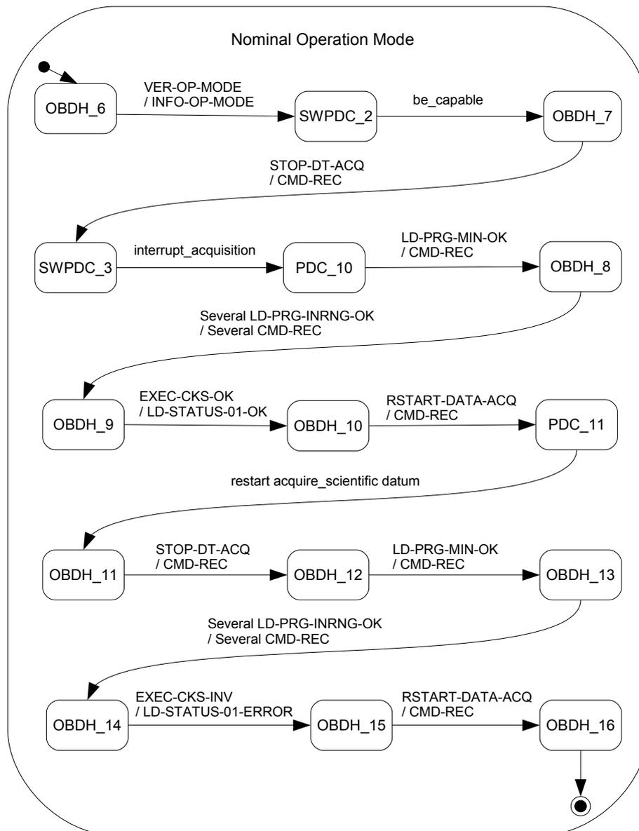
Figure 4.15 - SOLIMVA's unfolded scenario 109.3: *Nominal Operation Mode*
