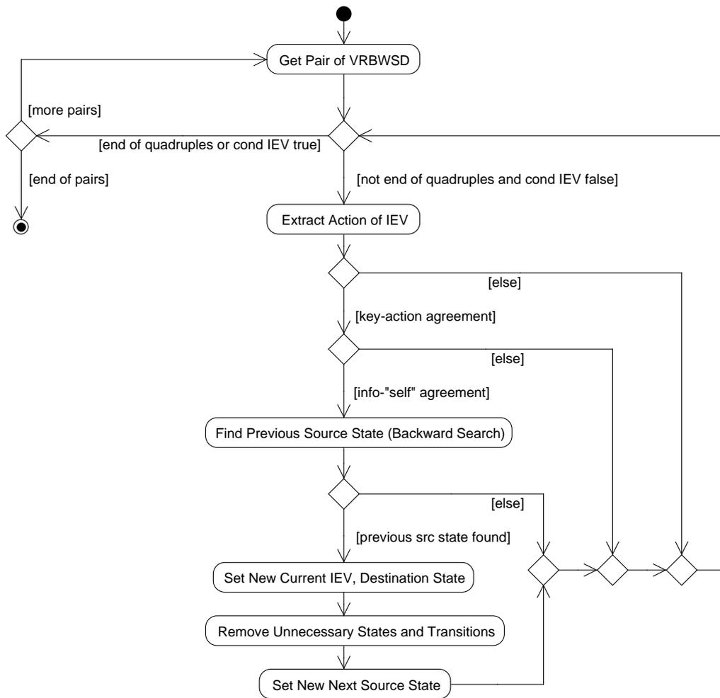
Figure 3.15 - Main WSD refinement algorithm: activity diagram
