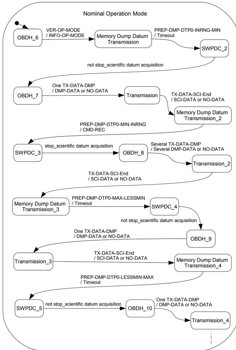
Figure 4.18 - SOLIMVA's unfolded scenario 73.2: *Nominal Operation Mode* (Part 1)
