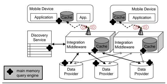
Figure 2: Architecture of a location-conscious data provisioning system integrating data from various providers
