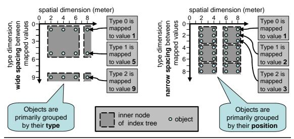
Figure 5: Effects of the spacing between mapped type values in the type dimension on the clustering of objects in the inner index nodes
