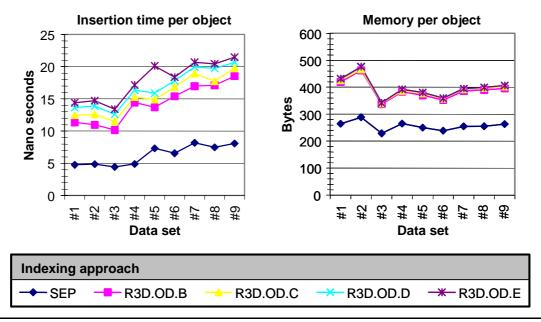
Figure 10: Average time for inserting a single object into the index, and average memory occupied by a single object (including geometry, bbox, type ID, and indexing overhead)
