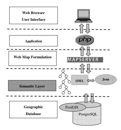
Figure 1. System Architecture with the Semantic Layer
