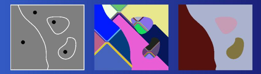
We want to propagate a distinct label for each minimum. This can be done by forcing a single root in each minimum.
