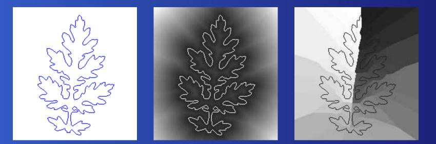
A consecutive integer number can be assigned to each contour pixel in S and propagated to the rest of the image.
