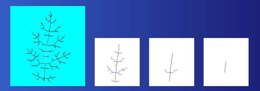
A difference image is obtained from the labeled image. Increasing thresholds create more simplified one-pixel-wide and connected skeletons.
