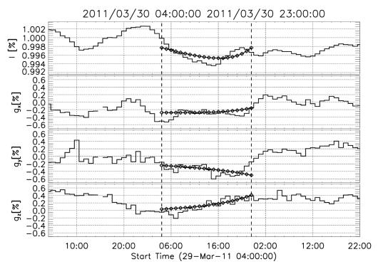
Figure 6.60 - The observation and modeling of cosmic ray depleted region associated to the magnetic cloud in 2011/03/30 using the conventional correlation system. The stair plot is the observed data and the line with diamonds is the modeling of the cosmic ray depleted region. The first panel, from top to bottom, shows the isotropic CR intensity. The remaining three plots show the orthogonal components of the fractional cosmic ray density gradient in the GSE coordinate system.
