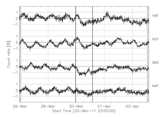
Figure 6.58 - The cosmic ray decrease observed by the vertical directional channels of the GMND during the MC on 2011/03/29. The vertical continuous lines correspond to the MC period suggested by the ICME catalog.
