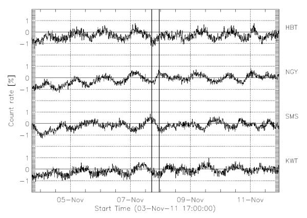
Figure 6.109 - The cosmic ray count rate observed by the vertical directional channels of the four muon detectors of the GMND during the MC at 2011/11/07. The two vertical continuous lines indicate the beginning and end of the MC.
