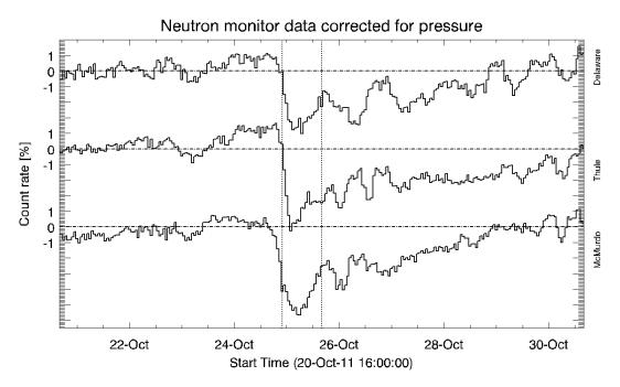
Figure 6.103 - The cosmic ray decrease observed by three different neutron monitors (Delaware, Thule and McMurdo) during the MC on 2011/10/25.
