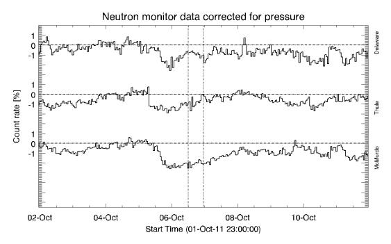
Figure 6.94 - The cosmic ray decrease observed by three different neutron monitors (Delaware, Thule and McMurdo) during the MC on 2011/10/06.
