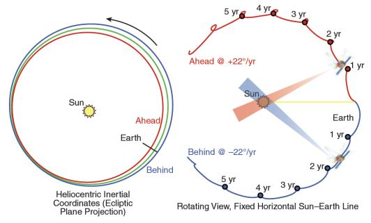
Figure 1.5 - The orbits of the twin STEREO spacecraft seen in the ecliptic plane by an observer located north of this plane. On the left, the trajectory is represented by an inertial Sun centered coordinate system. On the right, the Sun-Earth line (represented in yellow) is fixed to show the increasing distance from the Earth. Source: Dunham et al. (2009).
