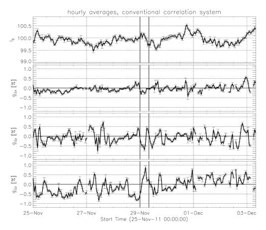
Figure 6.115 - The isotropic cosmic ray intensity and the orthogonal components of the cosmic ray fractional gradient during the MC period on 2011/11/29. The error bars indicate the error calculated from the six data points calculated using integration time of 10 minutes.
