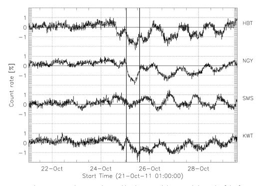
Figure 6.102 - The cosmic ray decrease observed by the vertical directional channels of the four muon detectors of the GMND during the MC on 2011/10/25.
