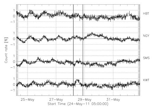
Figure 6.65 - The cosmic ray decrease observed by the vertical directional channels of the four muon detectors of the GMND during the MC on 2011/05/28.
