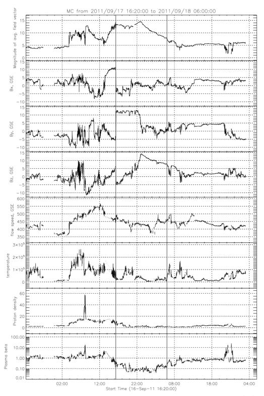
Figure 6.77 - The interplanetary magnetic field and plasma parameters during a MC on 2011/09/17. The vertical lines indicate the magnetic cloud timing.
