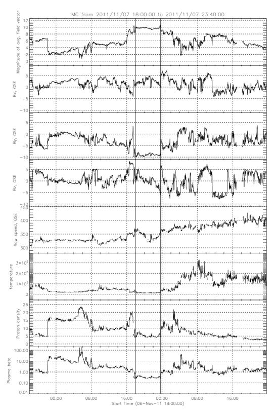
Figure 6.108 - The interplanetary magnetic field and plasma parameters during a MC at 2011/11/07.
