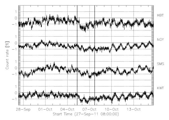
Figure 6.93 -The cosmic ray decrease observed by the vertical directional channels of the four muon detectors of the GMND during the MC on 2011/10/06.
