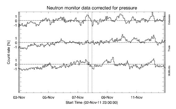
Figure 6.110 - The cosmic ray count rate observed by three different neutron monitors (Delaware, Thule and McMurdo) during the MC on 2011/11/07. The two vertical dashed lines indicate the beginning and end of the MC.
