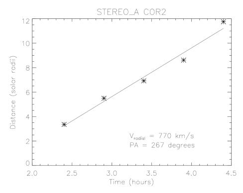
Figure 6.99 - The height-time profile of the CME on 2011/10/22 on the COR2A FOV for the fastest moving position angle. A linear fit is shown and the speed calculated in indicated. This CME was tracked by CORSET from 02:24 UT to 04:24 UT.
