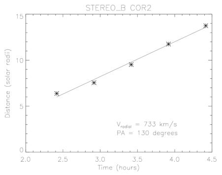
Figure 6.100 - The height-time profile of the CME on 2011/10/22 on the COR2B FOV for the fastest moving position angle. A linear fit is shown and the speed calculated in indicated. This CME was tracked by CORSET from 02:24 UT to 04:24 UT.
