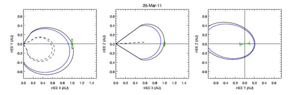
Figure 6.63 - The projection of the GCS model (represented in blue and black) and elliptical flux rope model (in green). For the former, the blue outline is the maximum measured height. The black outline is the model projected to the height when the front crosses Earth. The dashed line is the axis at the center of the cavity. Source: Colaninno (2012).
