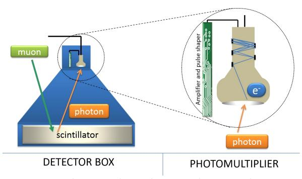
Figure 1.12 - Diagram of the internal configuration of a detection box for the detectors of the GMDN, except for Kuwait.
