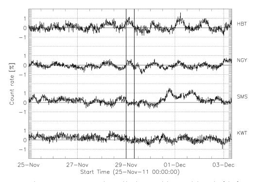
Figure 6.113 - The cosmic ray count rate observed by the vertical directional channels of the four muon detectors of the GMND during the MC on 2011/11/29. The vertical lines indicate the period of the magnetic cloud.
