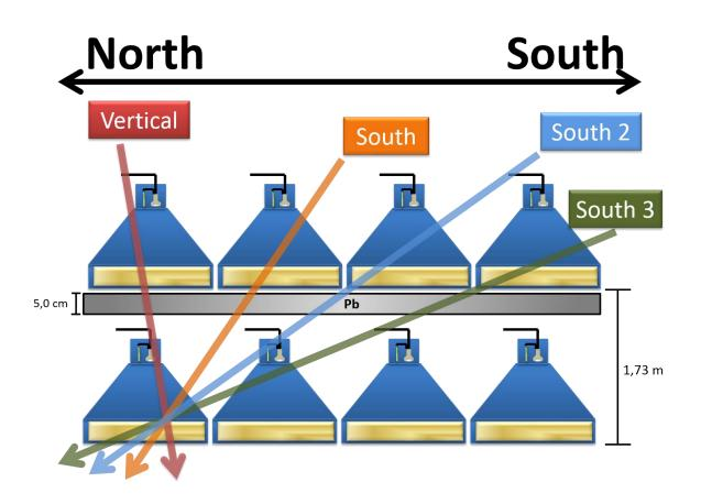
Figure 1.11 - A vertical cross section of a detector of the GMDN, except for Kuwait. Each detector is formed by two layers; each one has an array of detection boxes (Figure 1.12). In between the two layers, there is a 5 cm lead layer that absorbs the soft component of the cosmic rays. The four straight lines represent four samples muon arriving at the detector. Each of these muons will be computed in a different directional channel, as described in the text.
