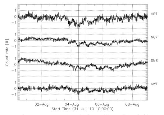
Figure 6.45 - The cosmic ray count rate observed by the vertical directional channels of the GMND during the MC on 2010/08/04.
