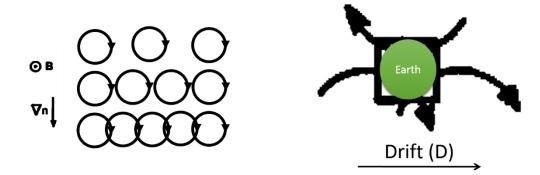
Figure 3.8 - The  $B \times \nabla n$  drift. Left side figure: each circle is a cosmic ray (positive charge) spinning due to the magnetic field B. The particle density at the top is smaller than in the bottom. Right side figure is a "zoom" of the scenario on the left; the 3 arrows indicate the 3 sample particles rotation. As there are more particles in the bottom, a current (drift) will be formed following the direction of rotation of the particles in the bottom.
