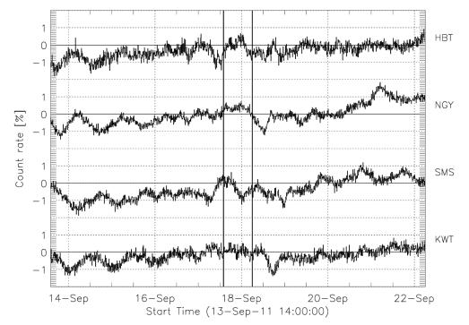
Figure 6.82 - The cosmic ray decrease observed by the vertical directional channels of the four muon detectors of the GMND during the MC on 2011/09/17.
