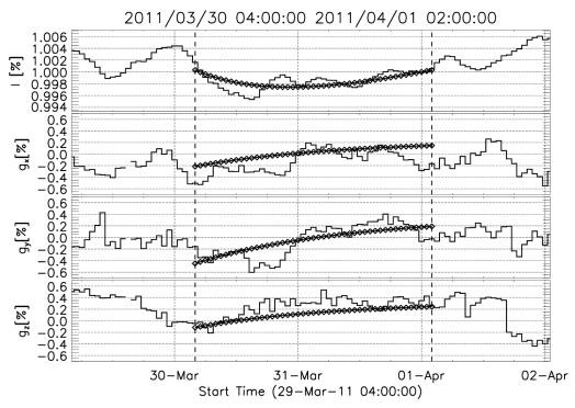
Figure 6.61 - The observation and modeling of cosmic ray depleted region associated to the magnetic cloud in 2011/03/30 using the conventional correlation system. The stair plot is the observed data and the line with diamonds is the modeling of the cosmic ray depleted region. The first panel, from top to bottom, shows the isotropic intensity. The remaining three plots show the orthogonal components of the fractional cosmic ray density gradient in the GSE coordinate system.
