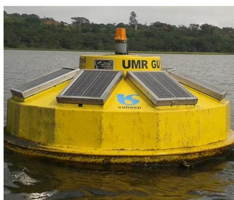
Adapted from Flores et al. (2001). Multi-parameter buoys installed in Guarapiranga reservoir.
