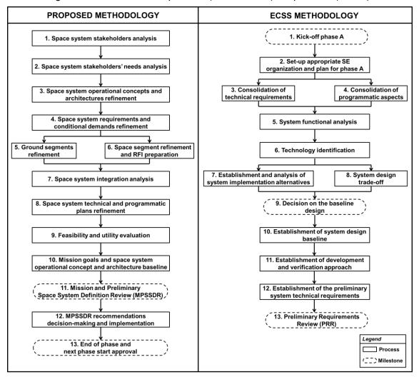
Figure 5.2 - Flowcharts of phase 2 (SPSYSE-TK) vs. phase A (ECSS).
