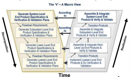
Figure 2.2 - The Vee model of systems engineering.
