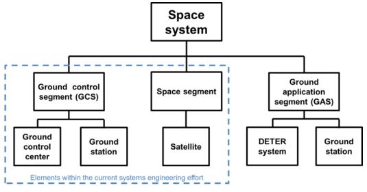
Figure 4.2 - Architecture for the space system concept #1 of the ARD-SM.
