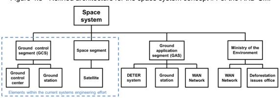
Figure 4.5 - Refined architecture for the space system concept #1 of the ARD-SM.
