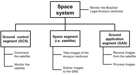
Figure C.4 - Space system architecture and main functions of each elements.
