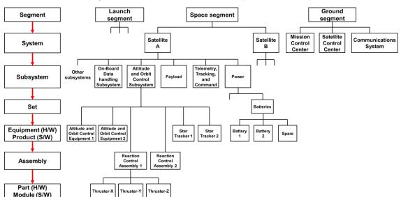
Figure 2.1 - Example of a space system hierarchy.
