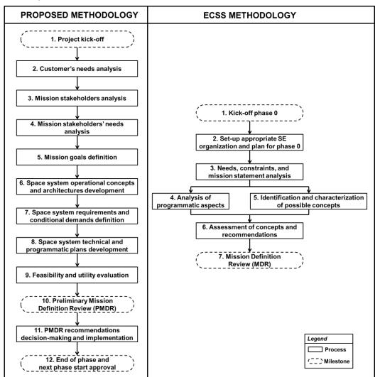
Figure 5.1 - Flowcharts of phase 1 (SPSYSE-TK) vs. phase 0 (ECSS).
