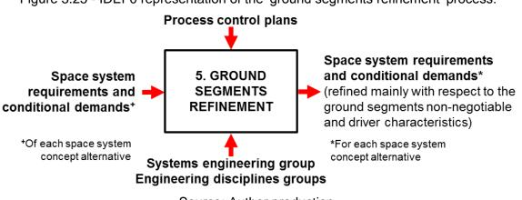
Figure 3.25 - IDEF0 representation of the 'ground segments refinement' process.
