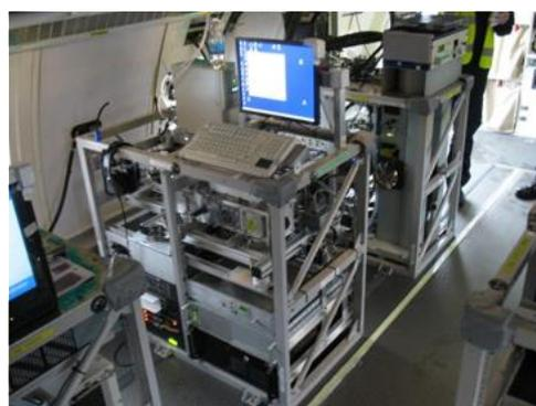
Aerosol Mass Spectrometry Rack
